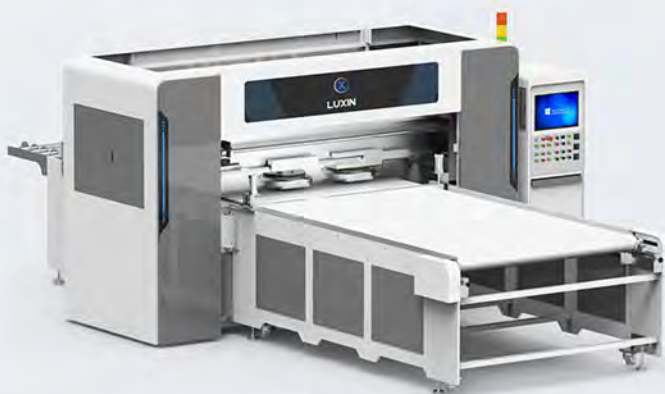
LX-125BK 快速双刀自动送料裁断机 FAST AUTOMATIC CUTTING MACHINE WITH DOUBLE KNIVES AND AUTOMATIC MATERIAL FEEDING MACHINE
