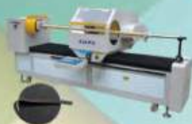
KAI-1126-SD 電腦全自動電腦分條機 Computer Full Automatic Cutting (Slitter) Machine
