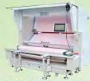
JN-887SRK-ED-2S 电脑控制针织圆型布双面验布机 COMPUTER CONTROLLED TWO-SIDED TUBULAR KNIT FABRIC INSPECTION MACHINE
